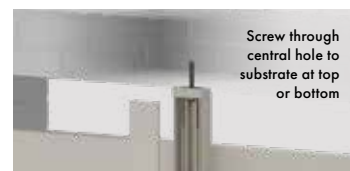
Screw top/bottom plate to centre support rail
